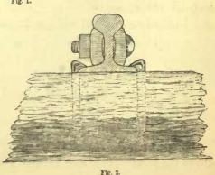
keeping the ends uniform in line and level. The fish-plates lie between the flange and head of the rail, and are only  $2\frac{1}{2}$  inches deep. As they have to endure the strain of passing trains, the rigidity of the joint is inferior to that of the rail, the latter having a larger sectional area and a depth of  $4\frac{1}{4}$  inches. The ordinary fish-plates do not, therefore, give perfectly unyielding joints.
